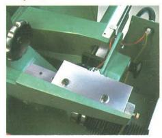
Cutters are ground in their block and old fashioned manual grinding is eliminated. The template ensures identical repeatability of cutter shape and profile.
