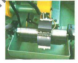
Cutter profile accuracy is guaranteed, and complex profiles from straight blanks can be produced very quickly, without having to allow for 'stretch' or 'development' on the template.
